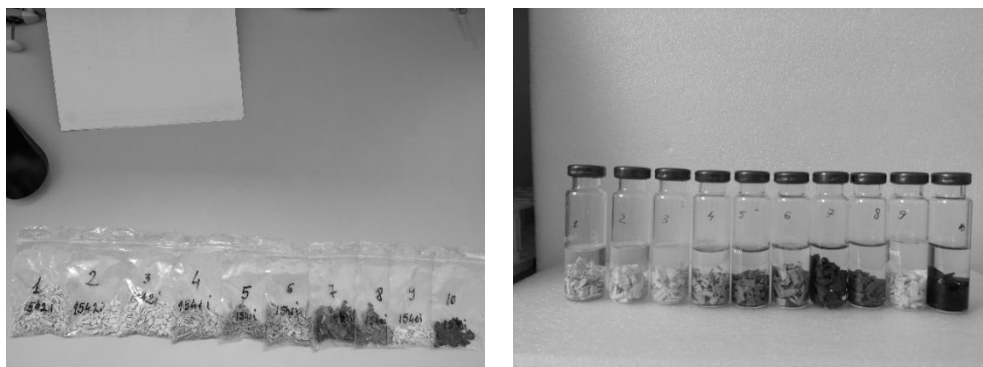
Figure 1. Chopped plastic materials (left) and Headspace extraction of volatile compounds from plastics (right)
